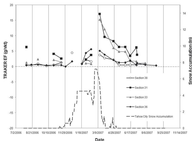
**Figure 5.** PM<sub>10</sub> road dust EFs of secondary road sections near Tahoe City SNOTEL station (missing data in the winter because of the sections covered by snow).
