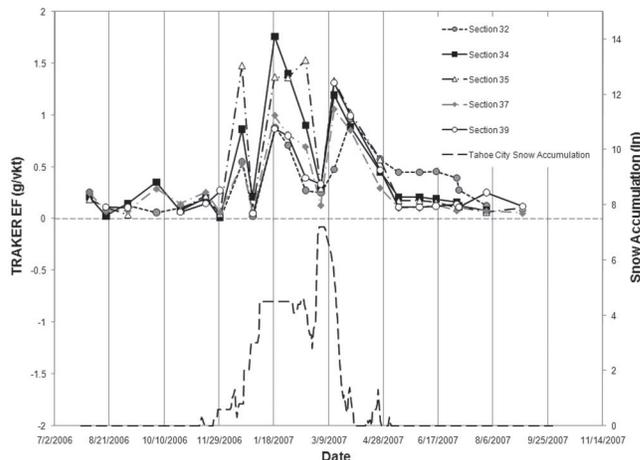
**Figure 4.** PM<sub>10</sub> road dust EFs of primary road sections near Tahoe City SNOTEL station.
