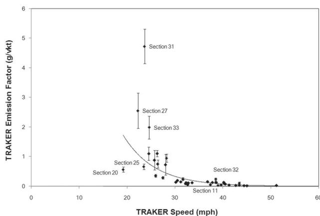
**Figure 6.** Relationship between TRAKER vehicle speed and measured average summer PM<sub>10</sub> EFs.
