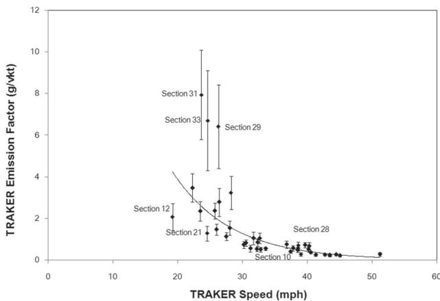
**Figure 7.** Relationship between TRAKER vehicle speed and measured average winter  $PM_{10}$  EFs.
