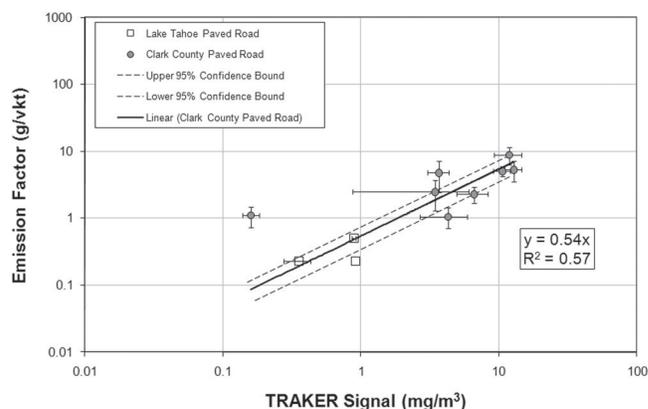
**Figure 1.**  $\text{PM}_{10}$  EFs vs. TRAKER average signal. Solid squares are data from the Boulder City, NV, study. The solid line represents a least-squares linear fit to the data from the Boulder City study with a zero intercept. The white squares represent data collected during an earlier study near Lake Tahoe, NV.<sup>27</sup> The dashed lines are 95% confidence bounds of the regression of Boulder City data.
